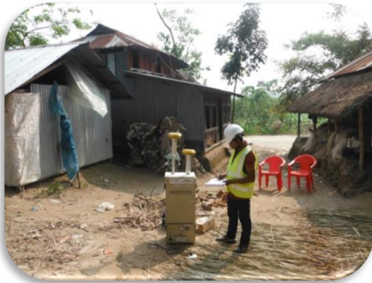
Ambient Air sampling at Nishanbari village
