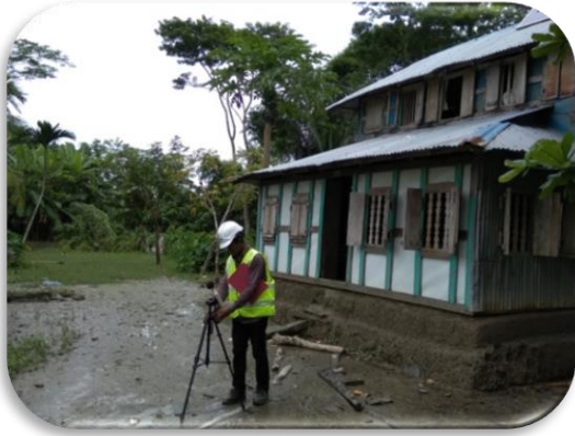
Noise Level Monitoring at Monir Hossain's House, Nishanbari village
